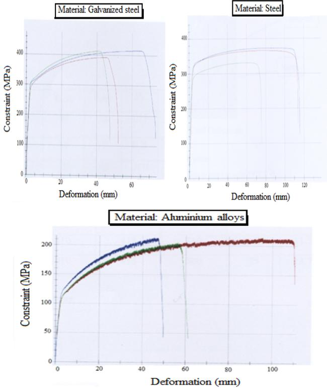
Fig. 1 Tensile curves for galvanized steel, aluminum alloys and steel
