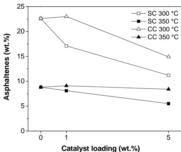
Fig. 2 C<sub>5</sub>-asphaltenes fraction from the cracking reactions as a function of catalyst loading (0% loading refers to thermal cracking)
