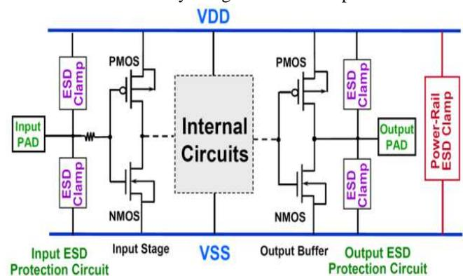
Fig. 1 The schematic of whole chip ESD clamp
