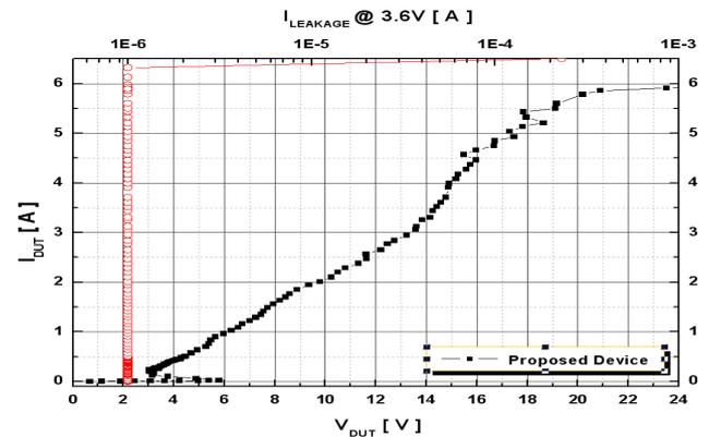
Fig. 6 TLP I-V characteristics of I/O ESD clamp device
