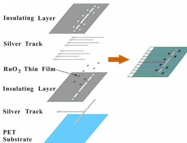
Fig. 3 Fabrication process of screen-printing  $2 \times 4$  sensor arrays
