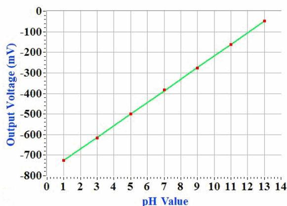
Fig. 7 Sensitivity and linearity of sample 8
