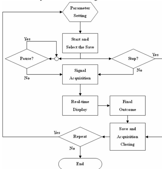
Fig. 4 Block chart of array measurement system
