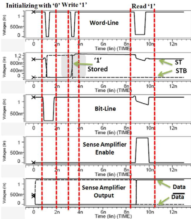
Fig. 4 Simulated waveform for writing '1' and read it
