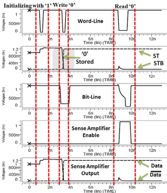
Fig. 5 Simulated waveform for writing '0' and read it
