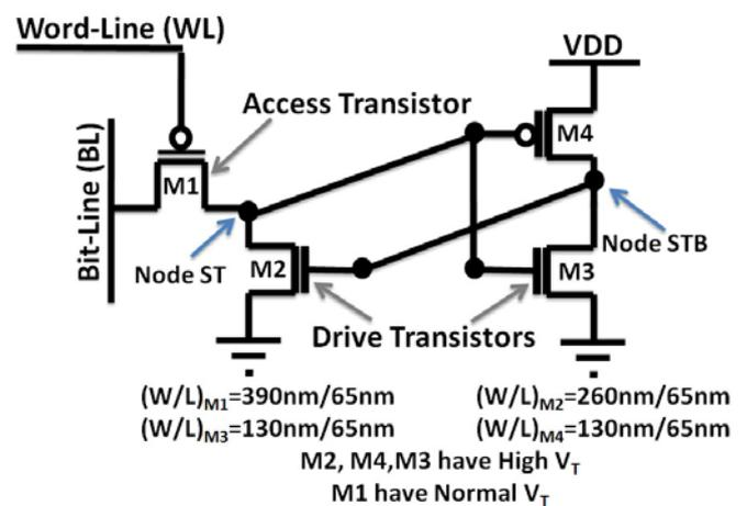
Fig. 1 Novel SRAM cell in 65-nm technology node.
