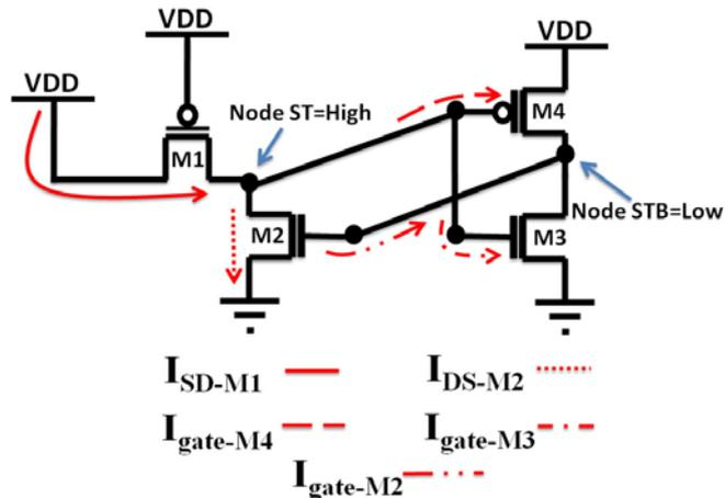
Fig. 2 Leakage current in idle mode when '1' stored in cell
