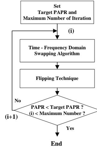
Fig. 5 Flow chart of proposed algorithm
