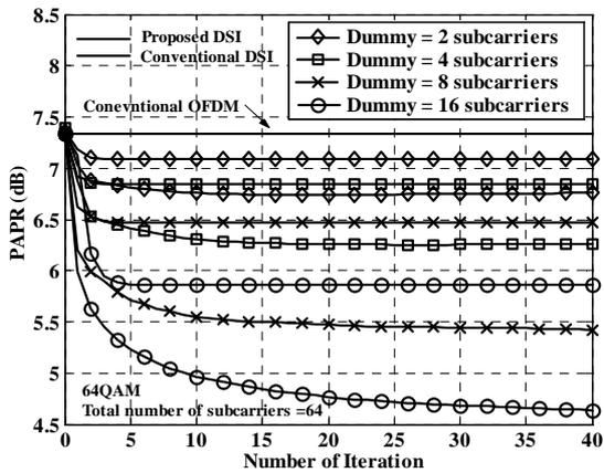
Fig. 7 PAPR performance versus number of iterations
