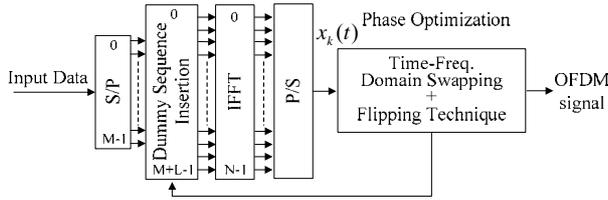
Fig. 4 Block diagram of phase optimization method
