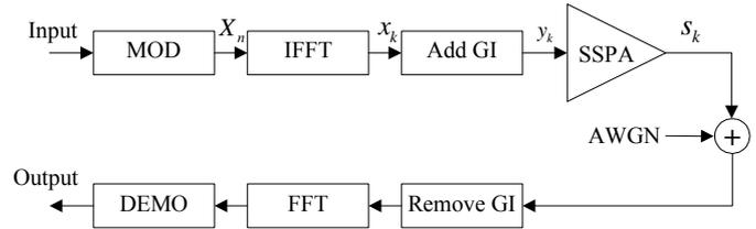
Fig. 1 Block diagram of OFDM system
