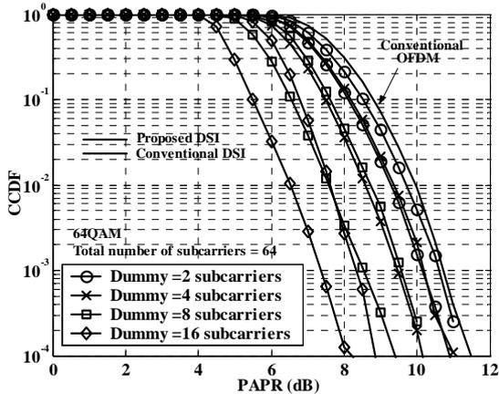
Fig. 6 PAPR performance of proposed DSI method
