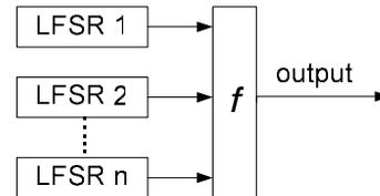
Fig. 2 Structure of combining generator
