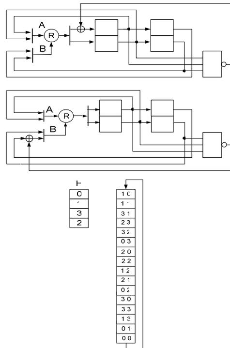
Fig. 11 Designs of RFSR with length  $2^n$
