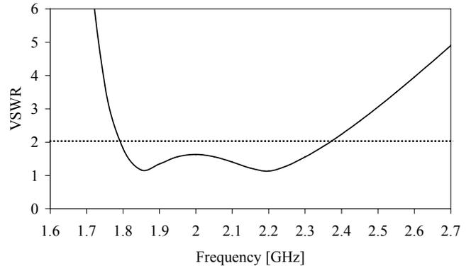
Fig. 2 Simulated VSWR of the proposed patch antenna
