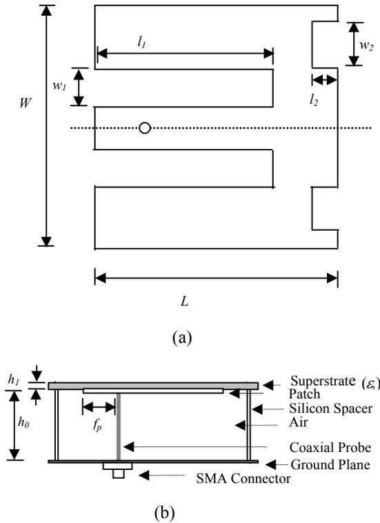
Fig.1 Geometry of proposed patch antenna. (a) Top view, (b) Side view
