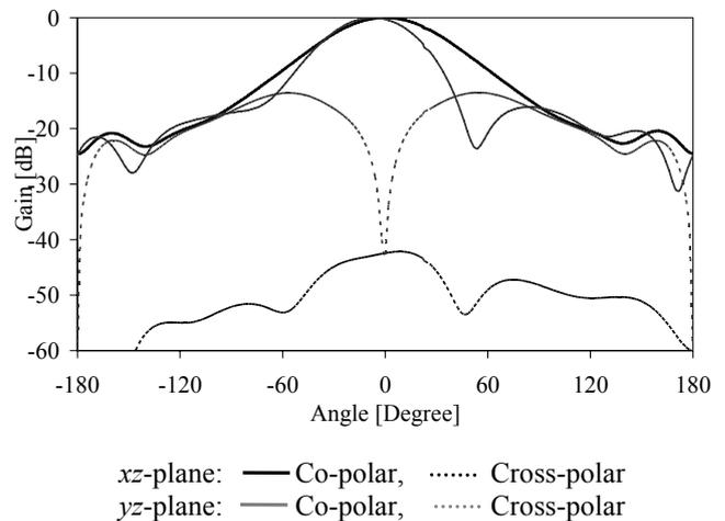
Fig. 3 Radiation pattern of proposed patch antenna at 2.2 GHz for  $xz$ -plane and  $yz$ -plane
