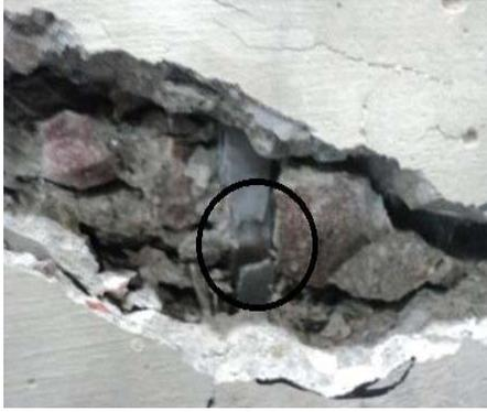
Fig. 5the necking phenomenon of steel strips
