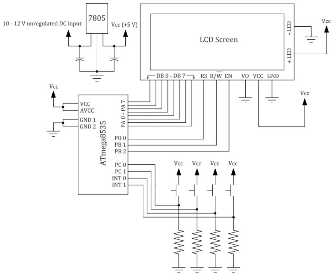
Fig. 7 Circuit diagram of the stop watch
