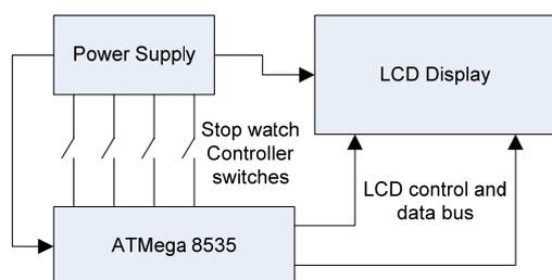
Fig. 1 Block diagram of the stop watch system
