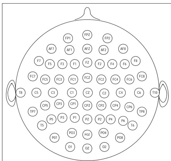
Fig. 1 61 channel electrode system
