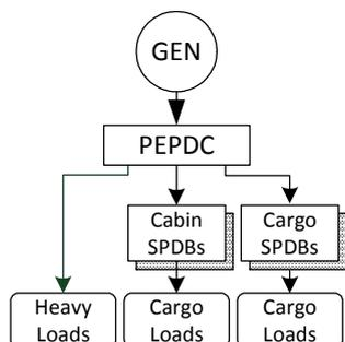
Fig. 6 Distributed Aircraft Electrical Power System [6]
