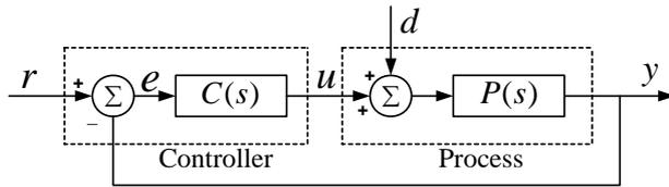
Fig. 1. Block diagram of basic feedback controller
