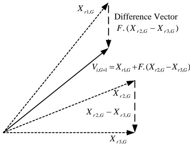
Fig. 3 Vector addition and subtraction in differential evolution
