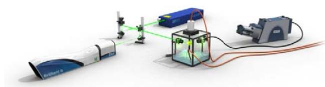
Fig. 1 LIBS system arrangement employing water jet
