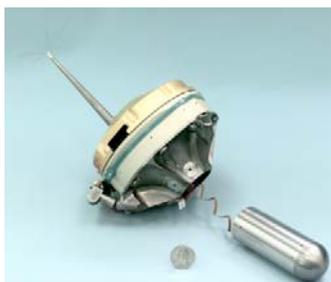
Fig. 1 Two body penetrator (DS2) [25]
