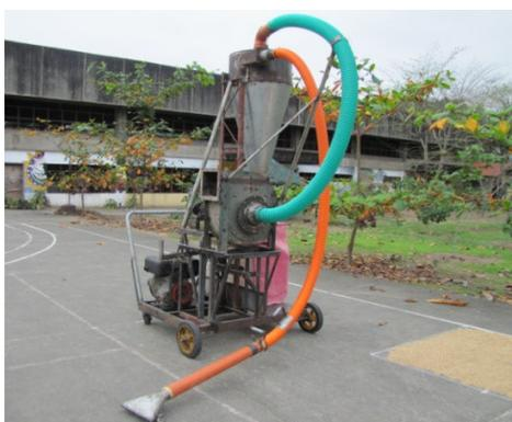
Fig. 2 Mobile engine-driven pneumatic paddy collector
