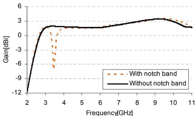
Fig. 6 Peak gain of the proposed antenna
