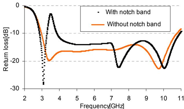
Fig. 5 Performance of the proposed antenna against frequency
