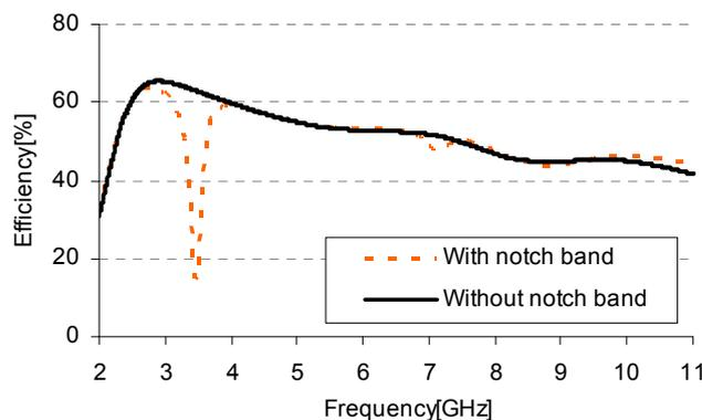
Fig. 7 Radiation efficiency of the proposed antenna
