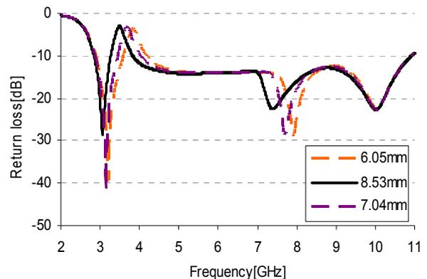
Fig. 3 Simulated return loss for different values of  $l_1$
