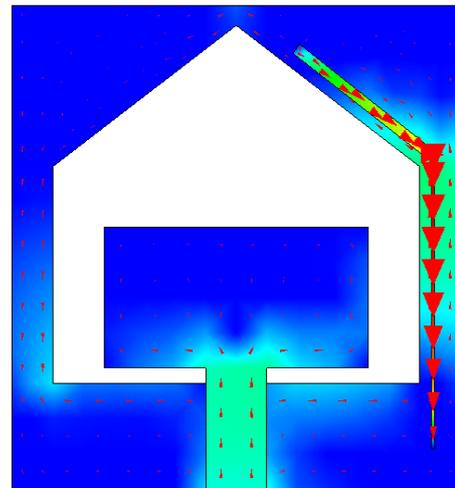
Fig. 2 Surface current distribution at 3.5 GHz
