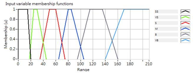
Fig. 9 Membership functions for the first input
