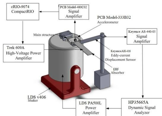
Fig. 5 Schematic diagram of semi-active vibration control architecture for a structure using the ER sandwich TVA
