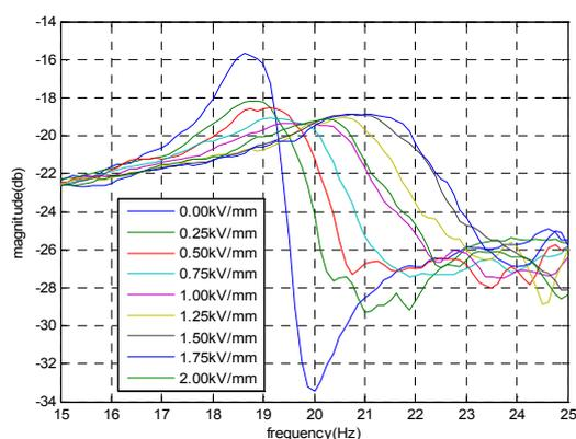
Fig. 6 The relationship between the frequency response (for the 1<sup>st</sup> mode) and the corresponding electric field (0~2 kV/mm)
