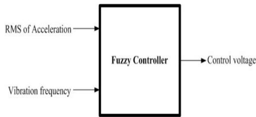
Fig. 8 The structure of the proposed fuzzy controller
