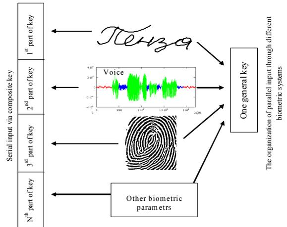
Fig. 5 Diagram of the formation of multi-biometric key code
