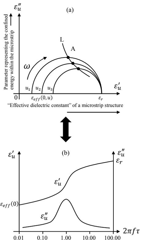
Fig. 3 (a) Cole-Cole representation of reactive relaxation of a microstrip structure with  $u = (w/\lambda)(h/\lambda)$  and  $u_1 < u_2 < u_3$
