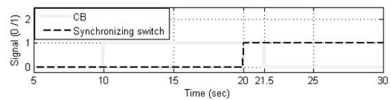
Fig. 17 Control signals for (CB and synchronizing switch)
