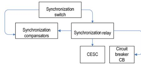
Fig. 5 Synchronization controller (SC)
