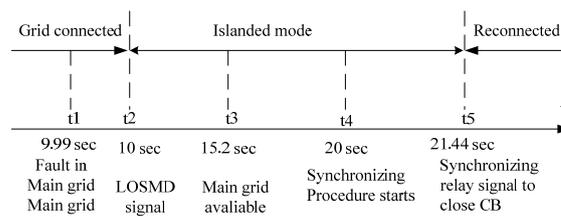
Fig. 24 Control system time sequence from simulation results
