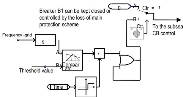
Fig. 4 Loss of main relay block diagram
