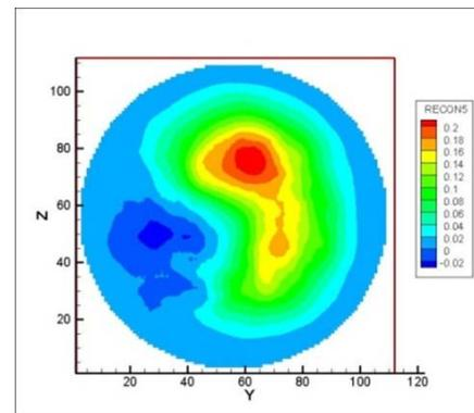
Fig. 4 Modes 1-2 axial vortex. Snapshot @ X = 320 mm
