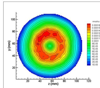
Fig. 2 Density RMS field. Snapshot @ X = 320 mm
