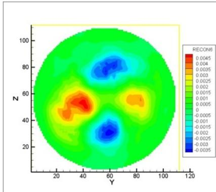
Fig. 5 Modes 3-4 transversal vortex. Snapshot @ X = 320 mm
