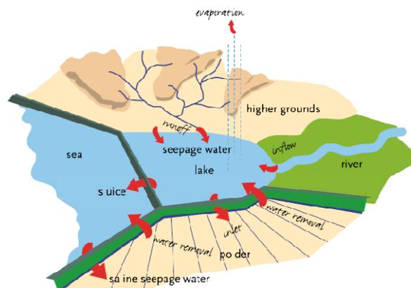
Fig. 2 The interconnectedness of the water system components [7]
