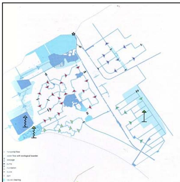
Fig 5 Circulation model applied in open water system in Almere [15]
