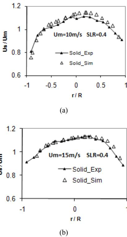
Fig.5 Comparison of normalized velocity curves.
