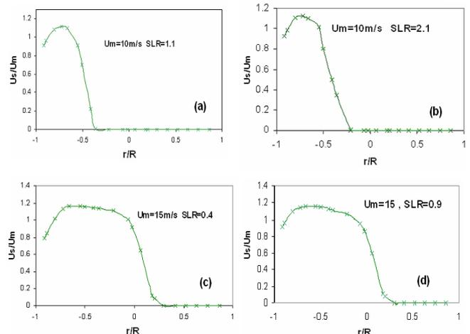
Fig.4 Velocity profiles of solid phase neglecting lift and particle-wall collision
