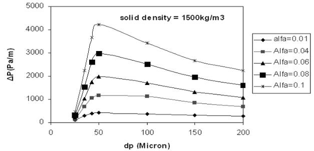
Fig.8 Effect of particle diameter on pressure drop for 30 mm pipe
