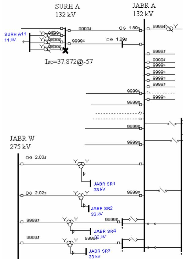
Fig. 3 A SLG fault at SURH A station
