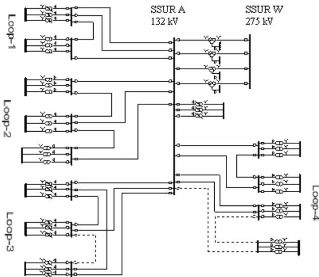
Fig. 2 Typical part of 132 kV network
