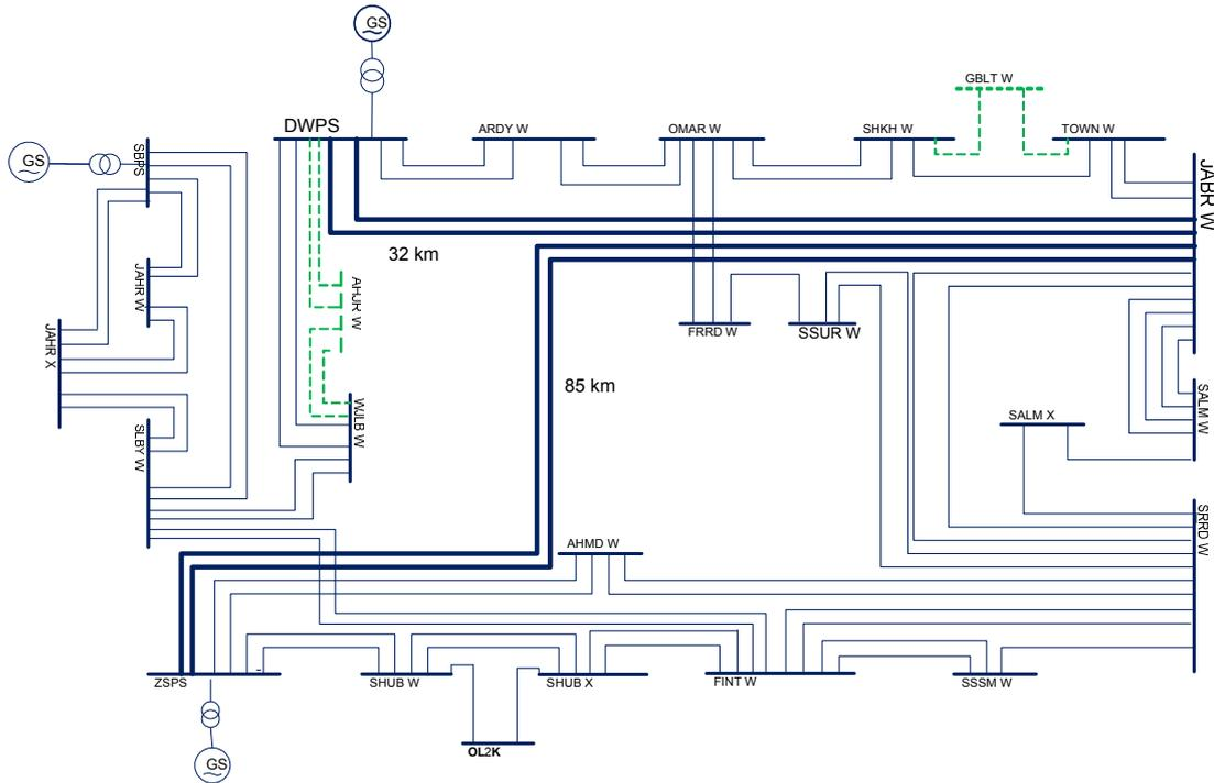
Fig. 1 The under study 275 kV transmission network
