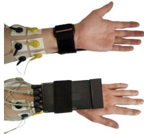
Fig. 4 Sensor modules and the EMG sensor attachment
