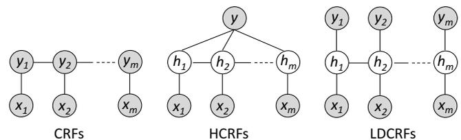
Fig. 1. Different type of discriminative models: CRFs, HCRFs and LDCRFs. In these models,  $x_j$  refers to the  $j^{th}$  corresponding observation value,  $h_j$  is a hidden states that assigned to  $x_j$ .  $y_j$  is the label of  $x_j$  where the gray circles represent the observed variables.
