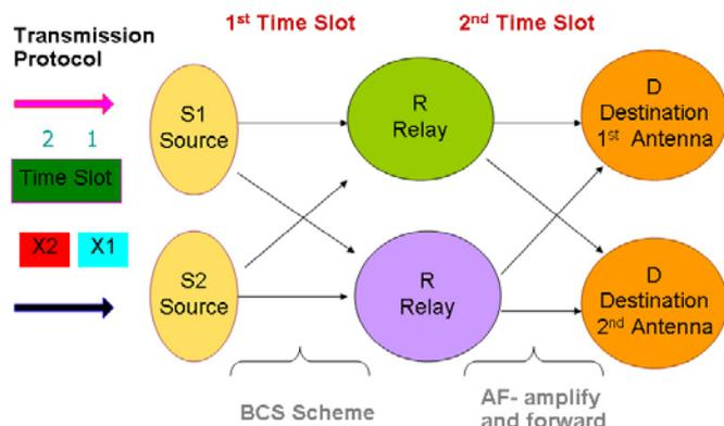
Fig. 1. Illustration of MIMO wireless network in Power and Cooperation Diversity gain mode with two source terminals  $S$ , two relays and the destination terminal  $D$  with two antennas
