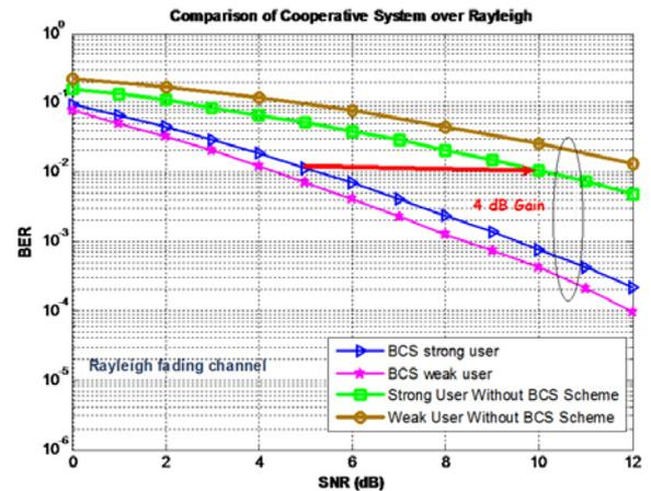
Fig. 7. The comparison of two-hop cooperative system between with and without BCS scheme
