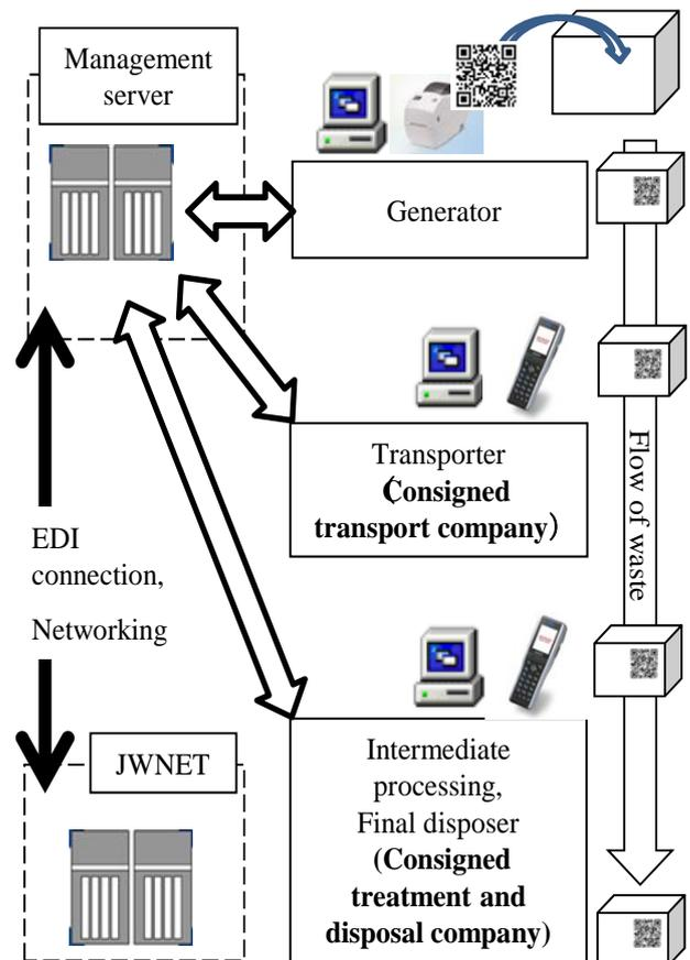
Fig. 1 Client server system developed by this research
