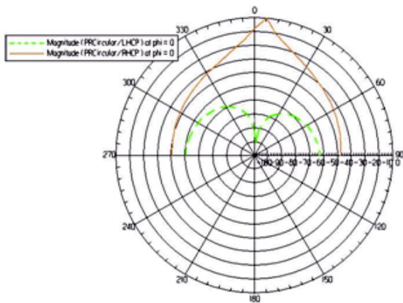
Fig. 5 Normalized polarization ratio versus theta at 1934 MHz
