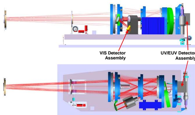
Fig. 2 METIS subsystems configuration, showing the position of the detectors assemblies (courtesy of Thales Alenia Space Italia)
