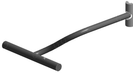
Fig. 3 Production fluid domain and valve cavity
