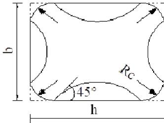
Fig. 3 Action of confinement for rectangular column
