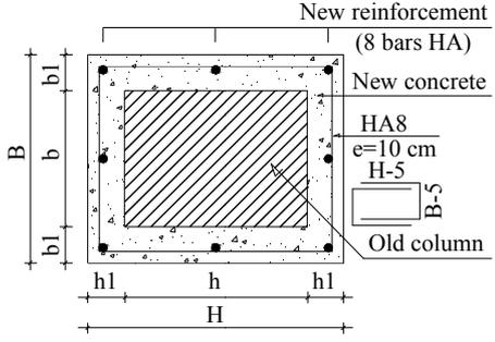
Fig. 2 Lining of column
