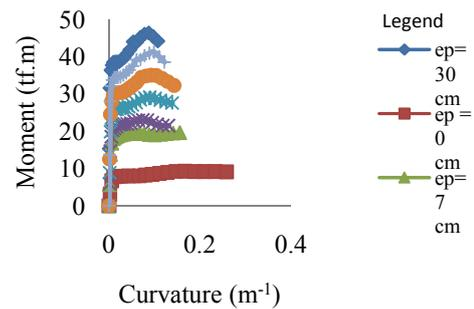
Fig. 9 Moment-curvature diagram for lined concrete sections
