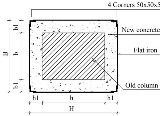
Fig. 6 Reinforcement brackets
