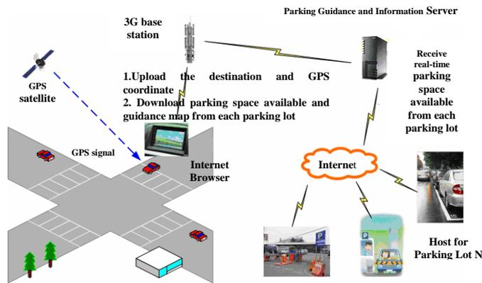
Fig. 2. An integrated architecture of Parking Guidance and Information System
