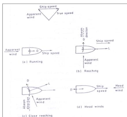
Fig. 2 Different modes of sailing (L and D denote lift and drag forces)
