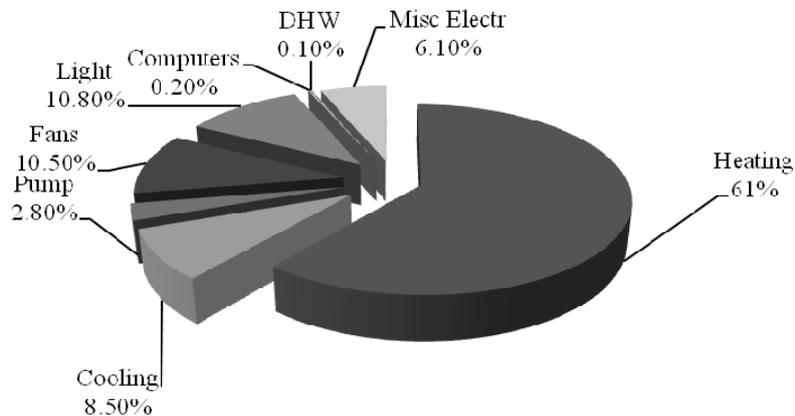
Fig. 2 CMLP Estimated energy breakdown in 2009 (UWO, 2010)
