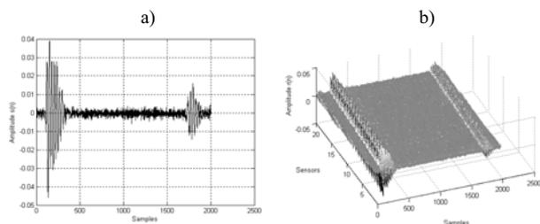
Fig. 2: Two buried targets example. (a) The selected reference signal  $s(n)$ . (b) Time-sensors representation of Data 1.
