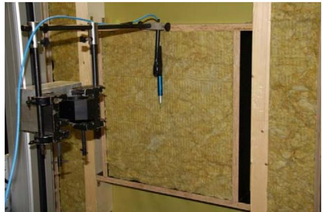
Fig. 6 Research on air flow-through velocity of mineral insulation by Experimental setup
