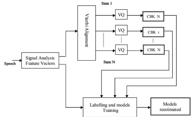
Fig. 3 Description of the training phase involved in the DVQ-HMM-based system
