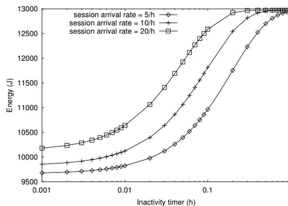
Fig. 3: Energy consumption by varying *inactivity timer*.
