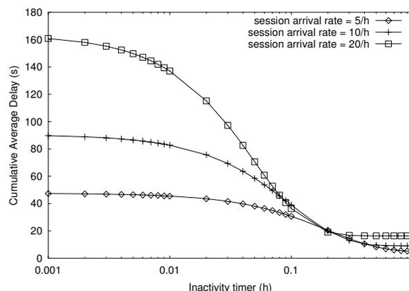
Fig. 4: Cumulative average delay by varying *inactivity timer*.
