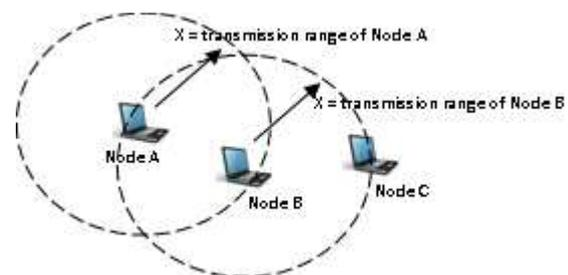
Fig. 1b Multi-hops (with 2 hops) where a destination node is out of source node's transmission range
