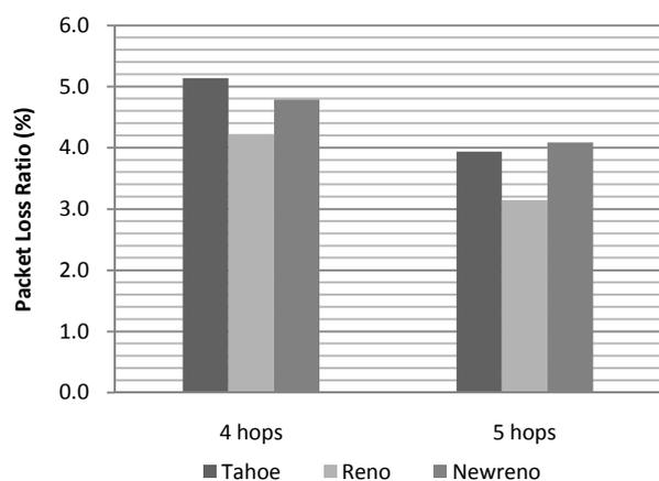
Fig. 10 Packet loss ratio for String topology
