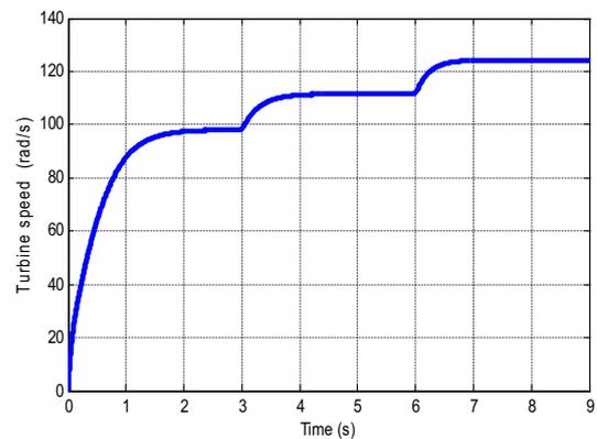
Fig. 5. Turbine speed according to the MPPT
