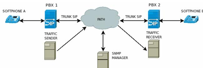
Fig. 4. Network testbed used for algorithm validation.
