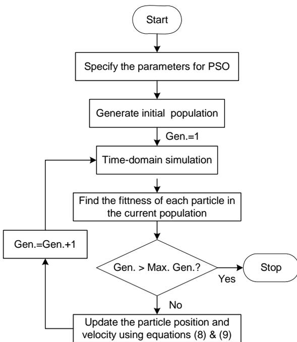
Fig. 5 Flowchart of particle swarm optimization algorithm
