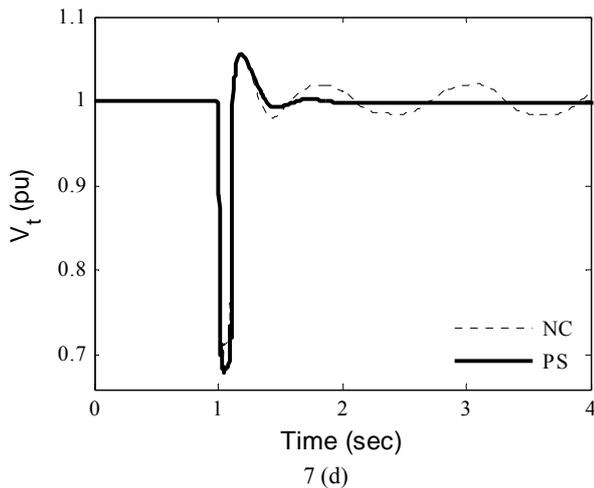
Fig. 7 System response for a 6-cycle 3-phase fault disturbance cleared by permanent tripping of one line. (a) power angle:  $\delta$ , deg (b) speed deviation:  $\Delta\omega$ , pu (c) line power:  $P_L$ , MW (d) terminal voltage:  $V_t$ , pu (e) SSSC controller injected voltage deviation:  $\Delta V_q$  (f) stator current: pu.
