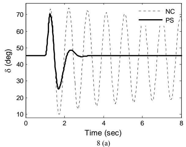
It is clear from the Figures that, the system is unstable without control under this severe disturbance. It can also be seen that, SSSC-based controller significantly suppresses the first swing in the rotor angle and provides good damping characteristics to low frequency oscillations by stabilizing the system much faster.
