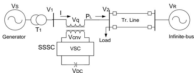
Fig. 1 Single-machine infinite bus power system with SSSC
