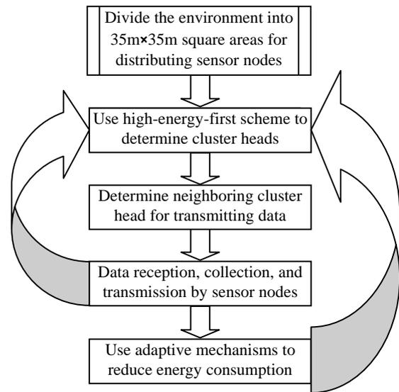
Fig. 4 The flowchart of dynamic routing method
