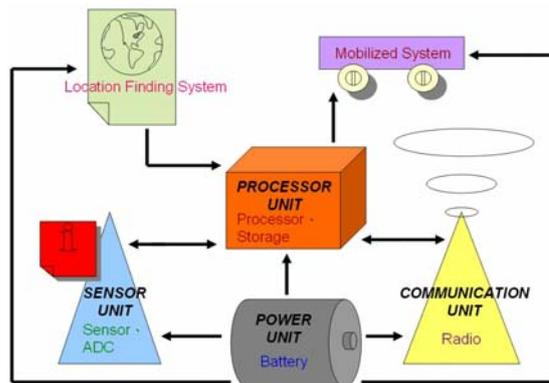
Fig 2. The basic units of a sensor device
