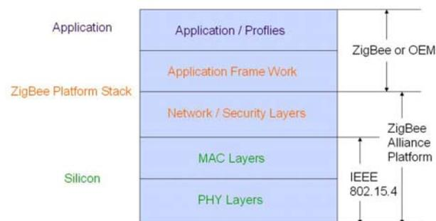
Fig 3. Combination of IEEE 802.15.4 and ZigBee protocols
