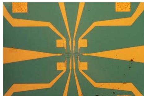
Fig. 1. Two transfer length measurement test structures each with 5 contact pads.
