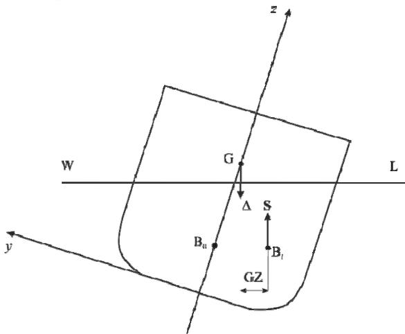
Fig. 1 Forces which act on any floating object.
