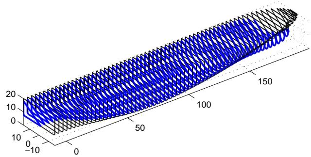
Fig. 2 Example of body hull input for Sectional Approach
