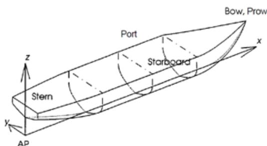
Fig. 7 System of coordinates according to DIN 81209-1 standard
