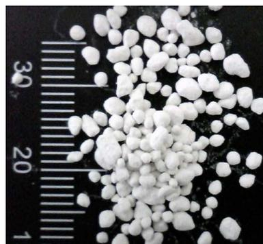
Fig. 1 Granules synthetic Zeolite NaA prepared influid bed metod
