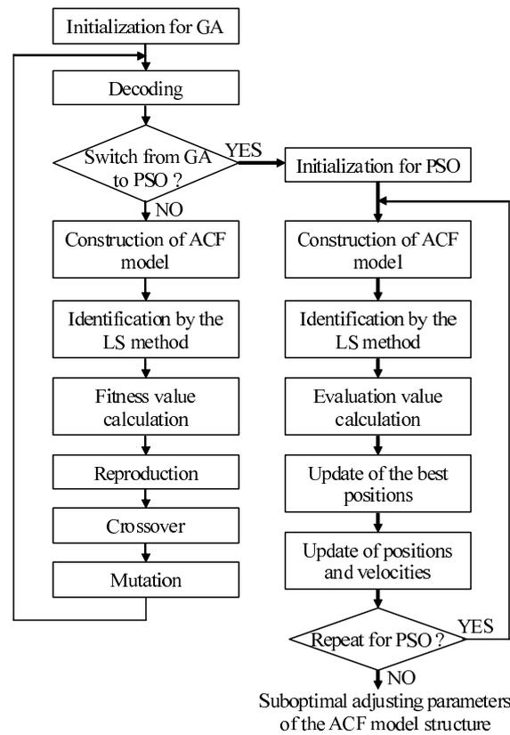
Fig. 5. Flow chart of the proposed hybrid method
