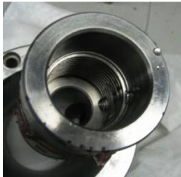
Fig. 7 Water droplets leaked deep in interconnect
