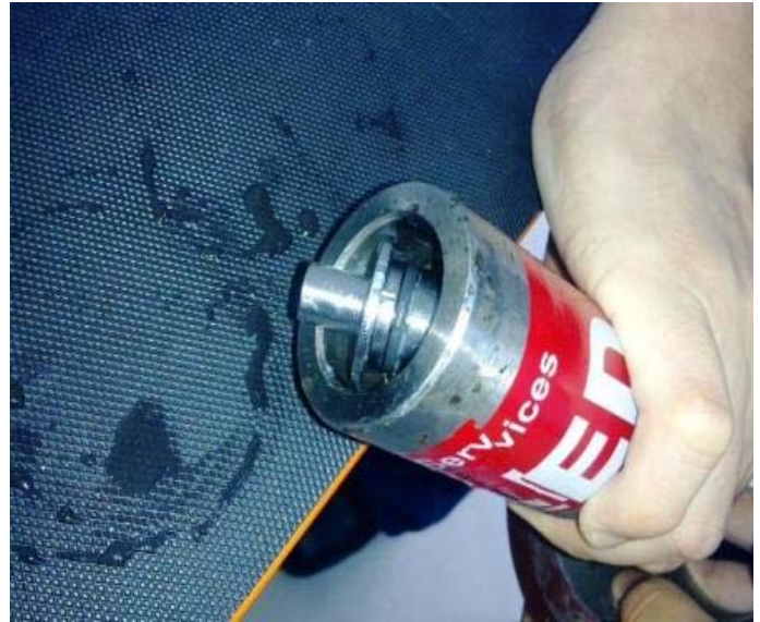
Fig. 3 Leakage inside the connector
