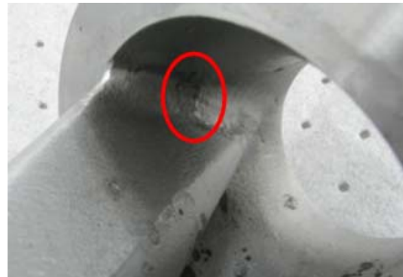
Fig. 4 Suspected casting defect area
