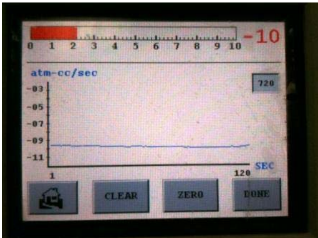
Fig. 5 Graph: Rate of Helium leak v/s time
