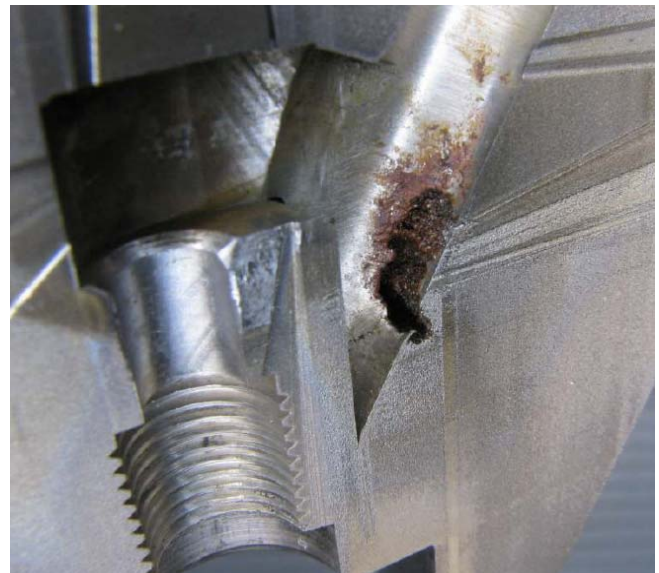
Fig. 9 Cavity found at defect location
